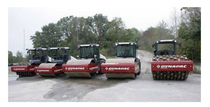
Tools: A fifth generation Dynapac CA soil compactor, equipped with Compaction Optimizer, incorporating Compaction Meter and Dyna@ Lyzer with GNSS (optional).
